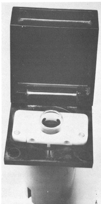
Fig. 2. Photograph of sample-cell positioner secured to sample cell and placed in sample-cell holder.
