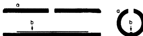
Fig. 1. Position of the graphite cloth ribbon in the graphite tube: (a) graphite tube; (b) graphite cloth ribbon.
